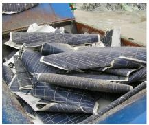
Solar energy generated by PV panels is a key element of the energy transition. However, the current discarding process of PV panels is still far from reaching high environmental and ethical standards. Today, most PV panels are either downcycled or landfilled and key raw materials are not recovered and therefore irreversibly lost.
